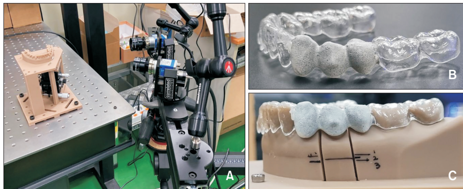
Figure 6. Experimental set-up for digital image correlation method. A , Images taken using two cameras; B , Clear aligner after speckle pattern coating; and C , Aligner mounted on the experimental apparatus.
